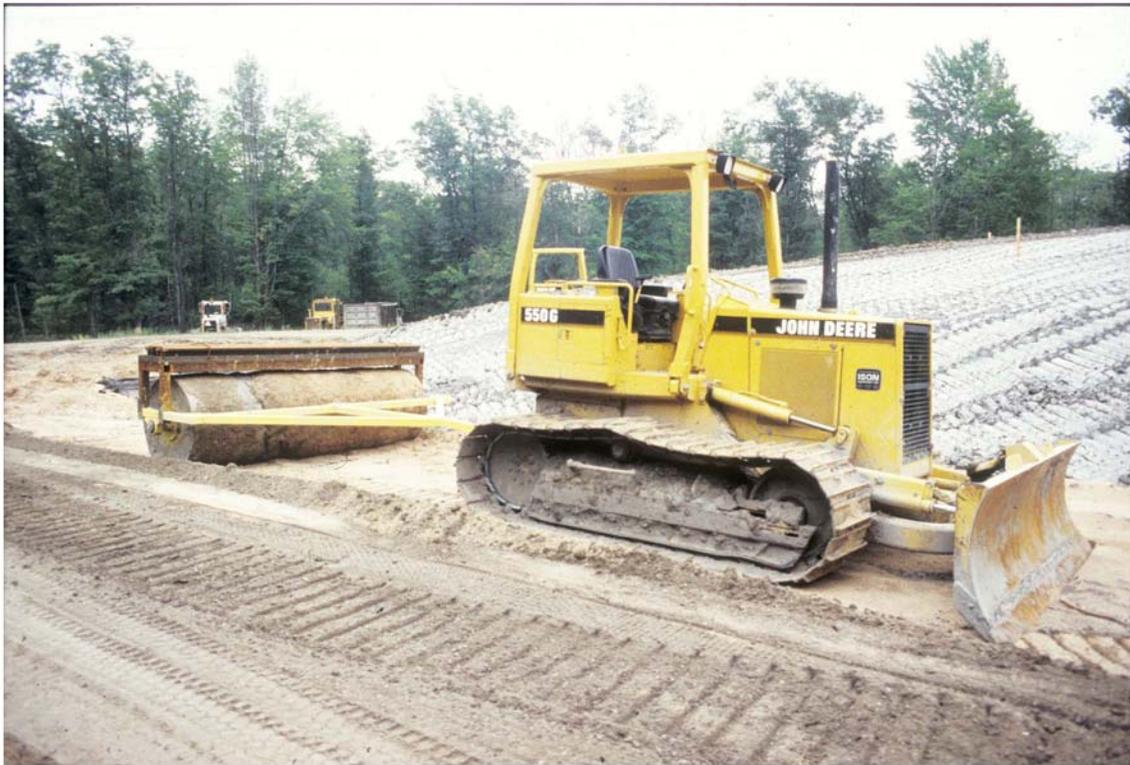
**Figure 3: Low Track Pressure Dozer with Smooth Roller. (From Maltby 2005, p-30)**
