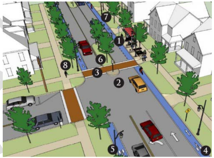
Image 13: Diagram of 'Complete Street', with opportunities for all transportation modes: pedestrians, bicyclists, bus riders and automobiles. www.localmotion.org
