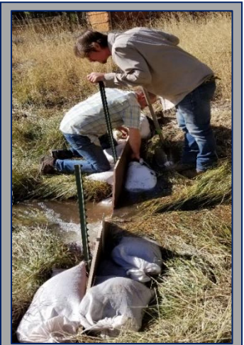
Weirs measure flows to determine seepage rates.
